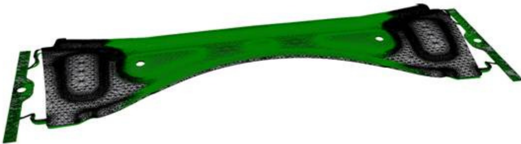
Fig 5. the topology-repaired original mesh and compensated mesh.
