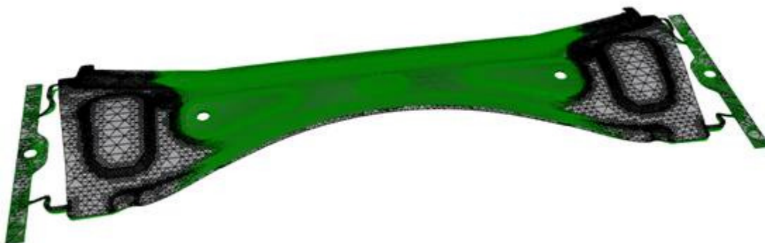
Fig2. the original mesh (in black) and the compensated mesh ( in green) created by spring-back simulation.
