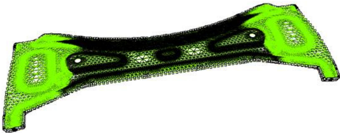
Fig 9. Boundary points are created in both original mesh and compensated mesh.
